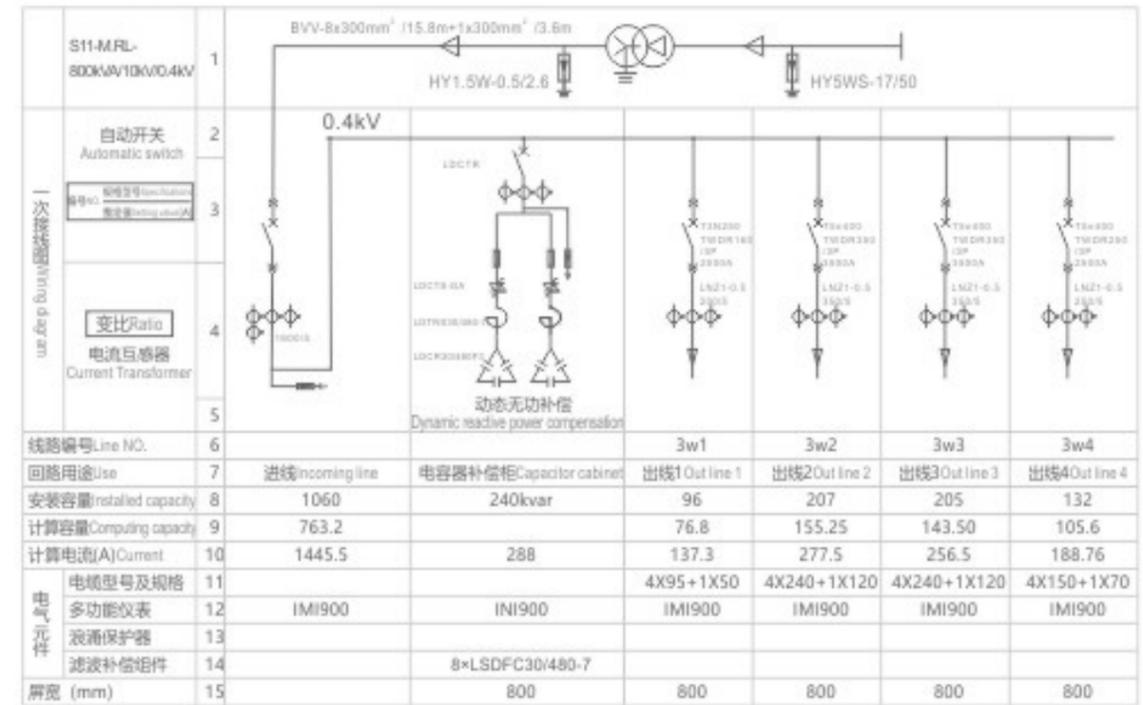
■ 静态无功补偿图纸设计 Static reactive power compensation design
