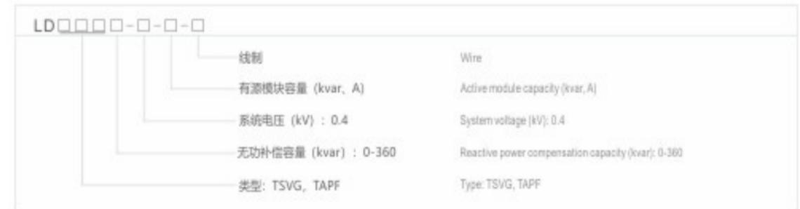
■ LDTSVG动态无功补偿图纸设计 Design drawing of dynamic reactive power compensation
